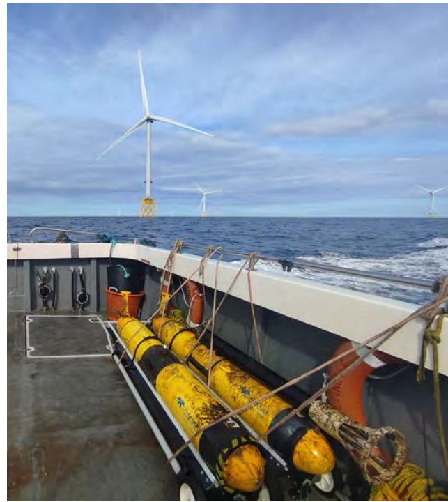
▲ Sluicm gliders recovered from the North Sea after quietly patrolling an area downwind of a major wind farm, off Scotland's east coast.
