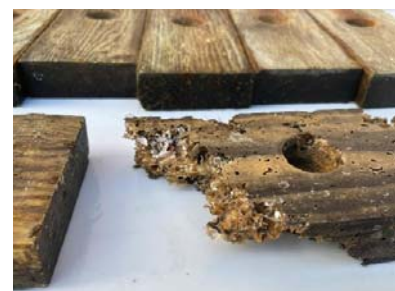
Shipworm damage in experimental wood
