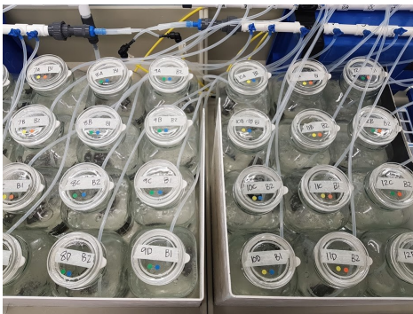
Experimental tanks aerated with an air/CO 2 mix to simulate end-of-century ocean acidification conditions.
