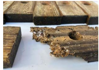
Shipworm damage in experimental wood
