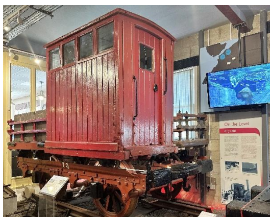
Two contrasting exhibits – Padarn Railway wagons (4ft gauge 'host wagon' conveying 1ft 10¾in slate wagons and guard's van), and model of the Awdry locomotive "Skarloey" derived from Talyllyn Railway No 1 "Talyllyn"
