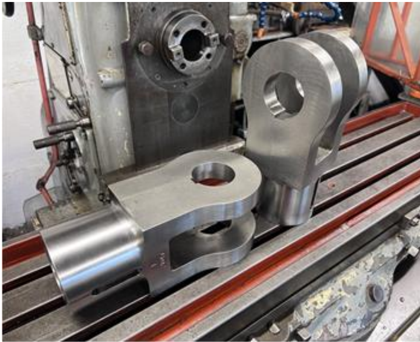
0-6-0ST MW2047 Warwickshire New Crossheads @ SVR Bewdley 12.1.25 (photo: Brian Hill)
