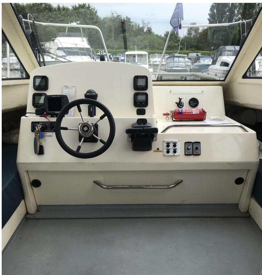
Boat helm showing clear space for wheelchair access.
