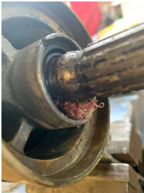
Port outboard motor propeller shaft – fishing line damage!
