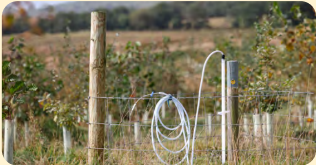
September 2022: A lysimeter helps to collect soil pore water samples at root depth
