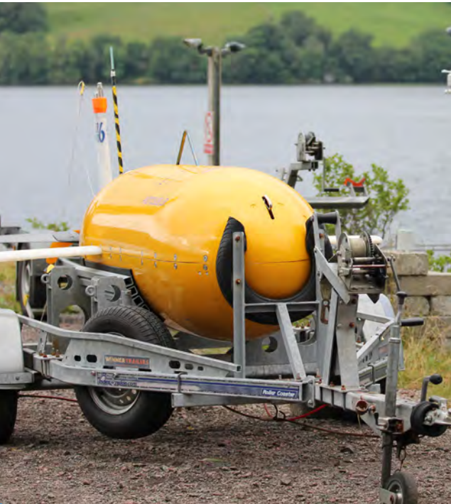
Autosub Long Range being prepared for under-ice capability testing in Loch Ness
