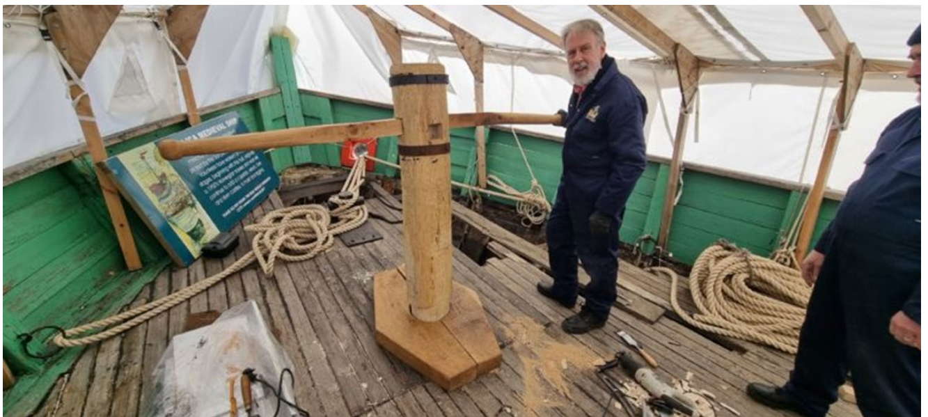
Capstan installed at deck level
