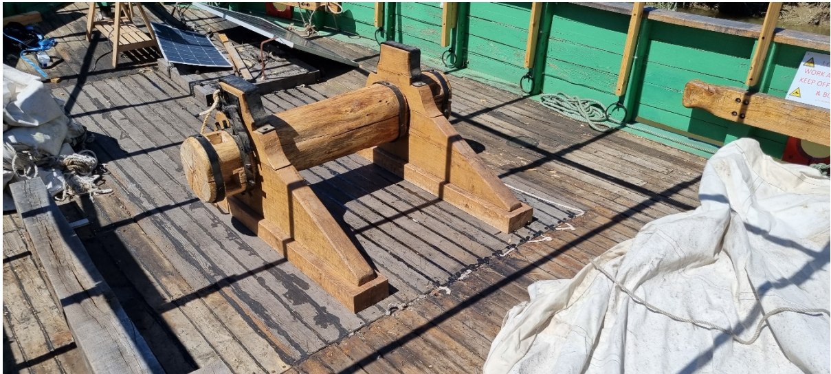
Windlass made in the Centre now in place
