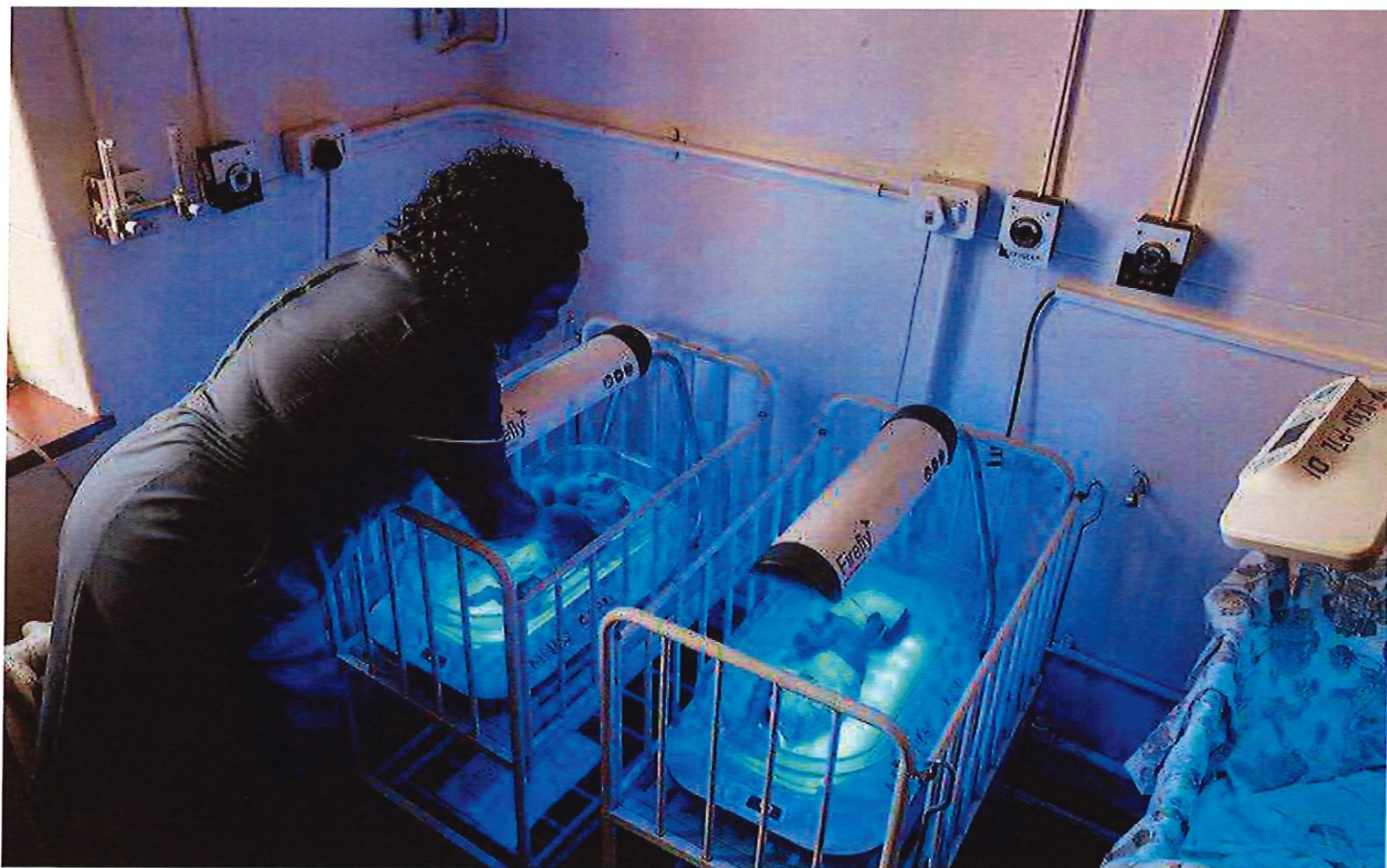
Firefly Phototherapy Device in use for jaundice management in the Mpilo Hospital Neonatal Intensive Care Unit
