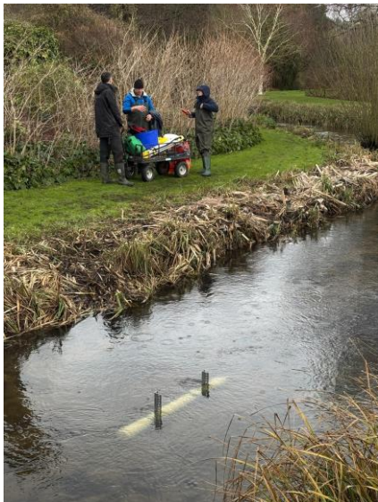
Installing a sediment collecting tube
