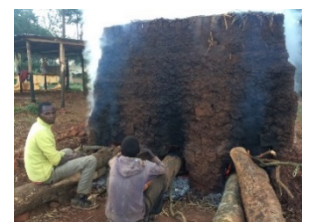
Traditional brick firing using tree trunks Credit: KEEP
