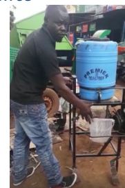
Foot-pedal Handwashing Station manufactured locally to our design Credit: KCWCG
