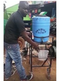
Foot-pedal Handwashing Station manufactured locally to our design Credit: KCWCG
