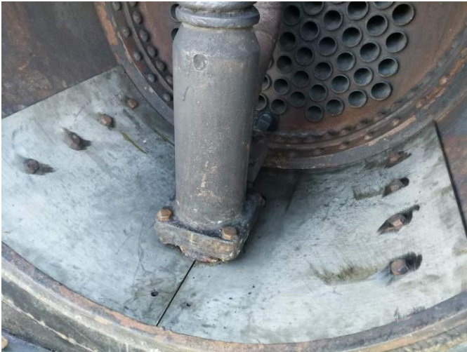
Gelert's new smokebox floor (left) and baffle plate (right) being made and fitted by our trustees and volunteers. (photos: Myles Jones)
