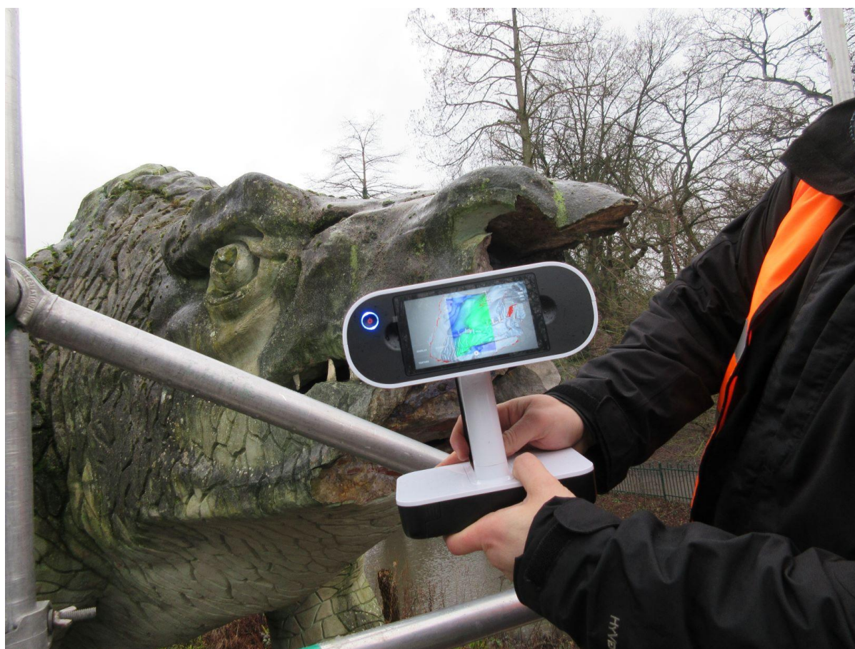
Figure 4: Scanning the exposed surfaces to design a close fit for the prosthesis. © Friends of Crystal Palace Dinosaurs
