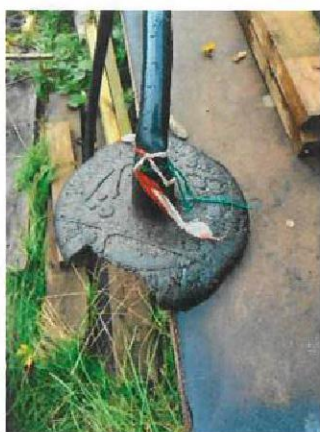
Damaged zip wire swing seat.
