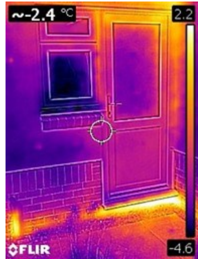
Infra red image showing heat leakage
