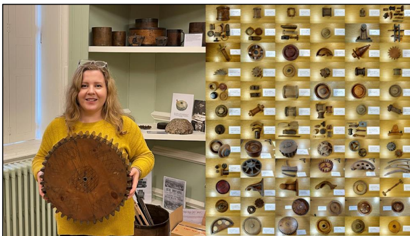
Director, Elizabeth Bartram, demonstrating one of the unique millwrighting patterns created for foundries to cast precisely engineered components of mill machinery. The display on the right captures part of the extensive collection built by Alan Stoyel over more than 60 years.
