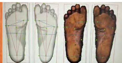
Sample 3D scans which are used to manufacture bespoke orthopaedic shoe insoles for patients which prevent Diabetic Foot Ulceration
