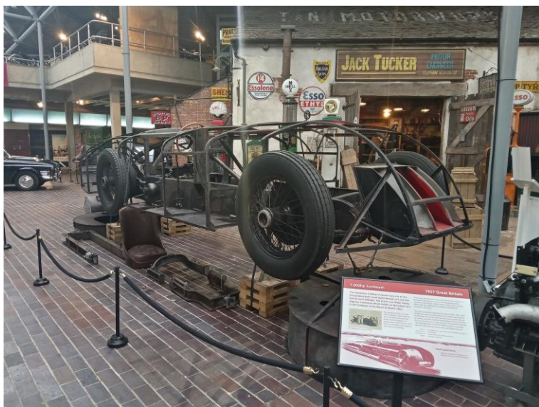
1927 1000hp Sunbeam in the Museum with body panels removed.
