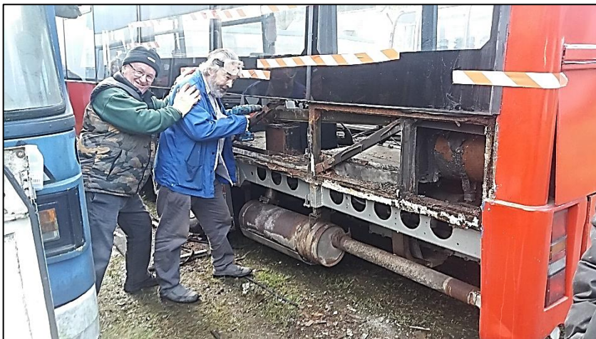
Volunteers remove body panels off Leyland Lynx F251 JRM prior to the rotten body frame being rebuilt.
