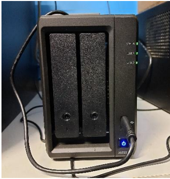
Network Attached Storage (NAS)
