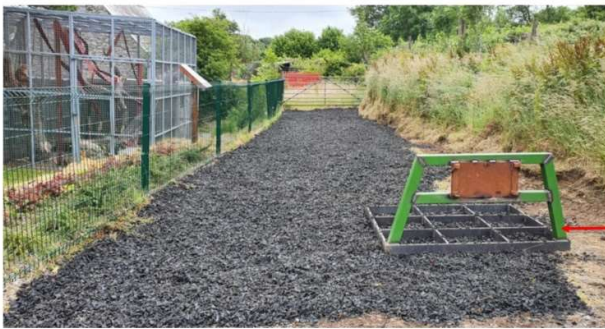
Graham made attachment for spreading rubber to fit on the back of the machine.
