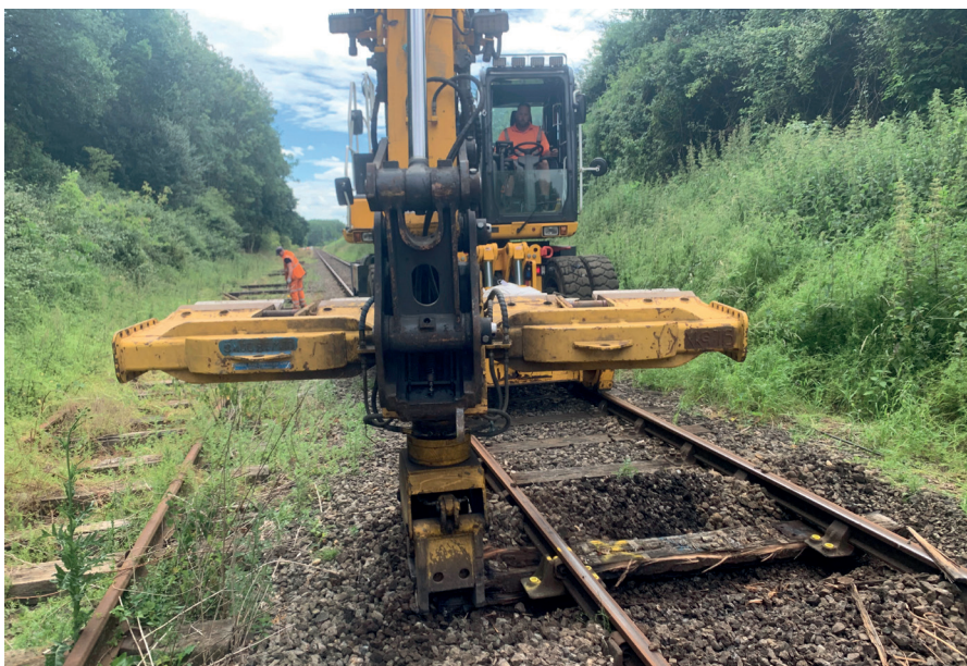
A Road-rail vehicle (RRV) for changing sleepers on this section. (PAUL THOMPSON)
